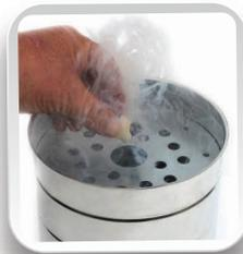
Drop 1 smoking pellet into generator though centre hole in disc
